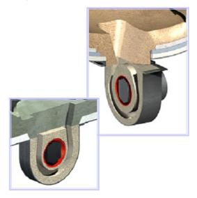
Kellundite for aluminium melting channel furnace inductors is based on high quality alumina with an addition of silicon carbide for improved performance
