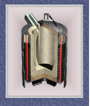
**Kellundite 395** - A spinel forming, 14% MgO lining based on chrome-alumina aggregate
